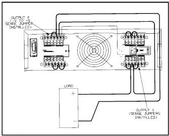
Figure 4-13. Series Connections with Local Sensing
